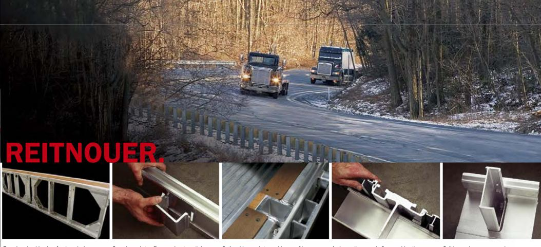
Two-piece load levelers for drop decks offer lighter weight handling and placement anywhere along the trailer deck.
